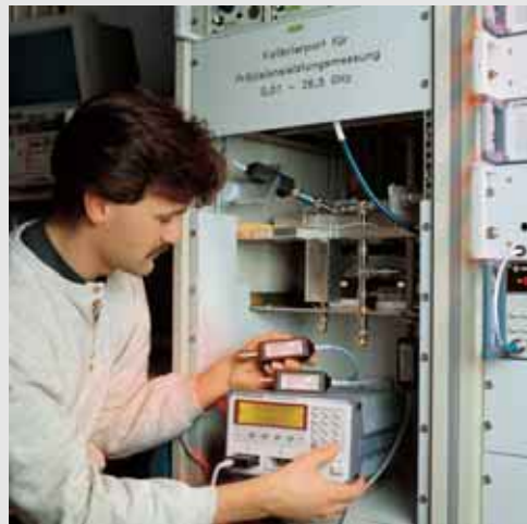
Calibration of the R&S ® NRV-Z sensors is directly traceable to the standards of the German Standards Laboratory
